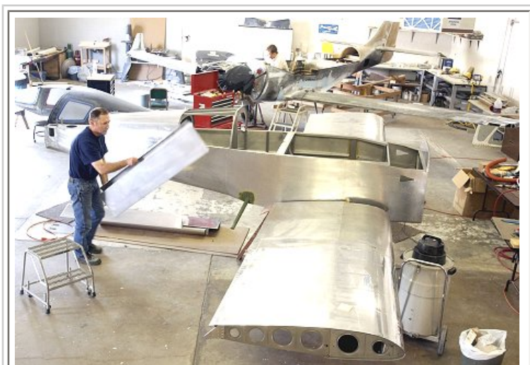
Builder's assistant Tom Meeker works on an RV-7 kit aircraft in the foreground as builder's assistant Isaac Nelson works on a Lancair IV-P kit in the background at Alpha Omega Aircrafters in SE Cedar Rapids on Tuesday August 17, 2004. The RV-7 is two-seater made from aluminum while the Lancair IV-P is a four seat pressurized carbon fiber aircraft. (The Gazette/Cliff Jette)
